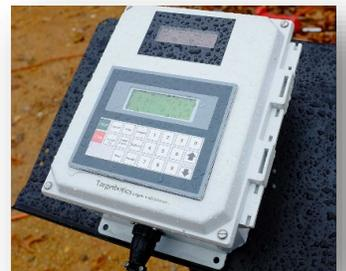
For the demonstration, Quitman mounted the OIT3185 in a small NEMA 4 enclosure and wired it up so that it would tick off numbers on the OIT. He then placed it in the bottom of a 5 gallon bucket of water for a week. The OIT worked perfectly, just as planned.
