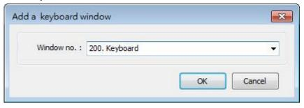
5. After the keyboard window is added, when you create Numerical Input and ASCII Input objects, "200. Keyboard" can be found in [Data Entry] » [Keyboard] » [Window no.]. The [Popup position] is for designating the display position of the keyboard on the HMI screen. The system divides the screen into 9 areas.
