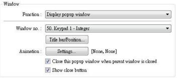
(cMT / cMT X Series) Animation Setting: cMT / cMT X Series allows using transition effects for opening popup windows using Function Keys. The settings can be opened by clicking [Animation Setting].
