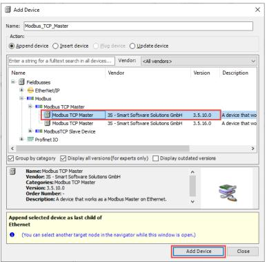
5. Select the new Modbus TCP Master device, then select Fieldbuses -> Modbus -> Modbus TCP Slave -> Modbus TCP Slave and click Add Device:
