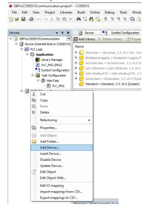
Select Fieldbuses -> Modbus -> Modbus TCP Master -> Modbus TCP Master and click Add Device:
