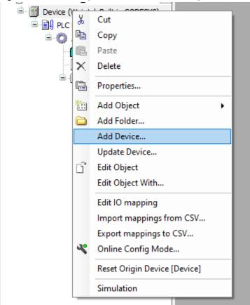
2. In the Add Device window, check the Display all versions checkbox and then select FieldBusses - > EtherCAT -> Master -> EtherCAT Master Version 3.5.10.0 and click Add Device:
