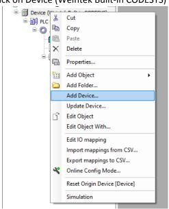
2. In the Add Device window, select Fieldbuses -> Ethernet Adapter -> Ethernet version 3.5.10 and click Add Device:
