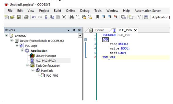
c. Right click on Application in the Devices pane and select Add Object -> Symbol Configuration, using the default values:
