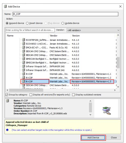
5. Select the newly added iR-COP device, and then in the Add Device window, add each module connected to the iR-COP in the order connected. In this example, we only have an iR-DM16-P connected:
