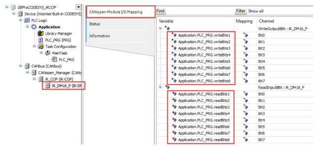
10. Still on the CANopen I/O Mapping tab, set Always update variables to Enabled 2 (always in bus cycle task).
