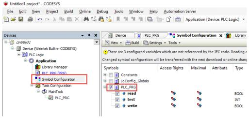
b. Select Build -> Generate Code to generate the XML file, which can be found in the project directory:
