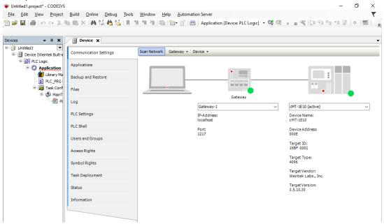
d. Note that it is also possible to simply type the IP address of the cMT-X device into the Scan Network tab device section:
