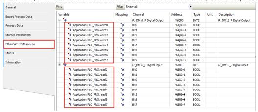
9. While in the EtherCAT I/O Mapping tab of the iR\_ECAT device, set the Always update variables to Enabled 2 (always in bus cycle task):
