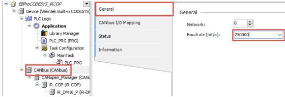
7. To map tags to the CANopen device, first add tags to the PLC\_PRG application. In this example, BOOL tags are used as the only IO module connected to the iR-COP is an iR-DM16-P:
