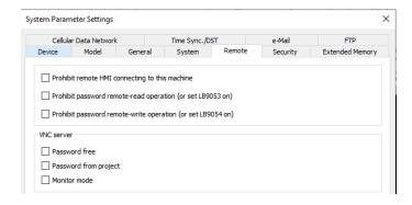
NOTE: It may be necessary to control the behavior and network access of the VNC feature. For more information, System Tags for VNC Control and Network Ports can be found below.
