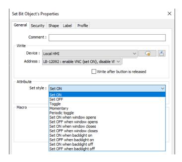
Once the Set Bit is placed and the project is downloaded to the HMI, VNC is now enabled. When opening VNC Viewer, the program will require a password. The default password is 111111.
