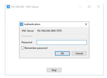
The password can be changed or bypassed in the System Parameters setting in EBpro under the Remote tab.
