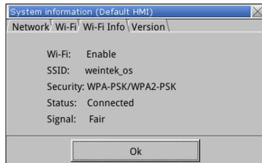
**Note:** When using the Wi-Fi simultaneously with the wired Ethernet port, ensure that the connections are on different subnets. Detailed instructions of the HMI5103L Wi-Fi capabilities are provided in **Tech Note 5121**, available from the Support Center of the Maple Systems website.
