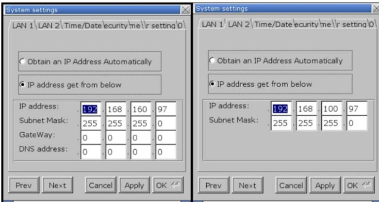
Notice in the above figure LAN1 is on the 192.168.160.xxx subnetwork, while LAN2 is on the 192.168.100.xxx subnetwork. For both ports to operate simultaneously, they must be assigned to different subnetworks.
