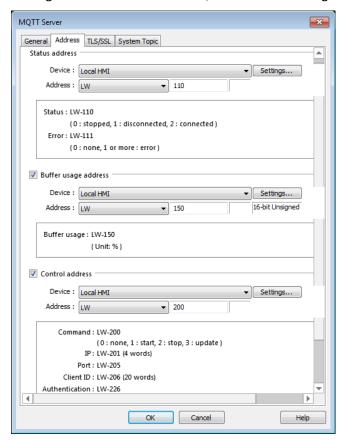
The MQTT\_COMMAND control addresses can be designated to set control parameters, and the corresponding addresses include MQTT\_COMMAND+1  $^{\sim}$  MQTT\_COMMAND+70...etc. The status addresses can show connection status, and the corresponding addresses include MQTT\_STATUS and MQTT\_STATUS+1.
