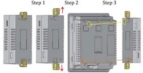
Step 1: Pull the two white lock connectors out from the center of the module.
